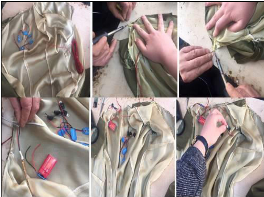
Figure 9. Integration of leds into the fabric
