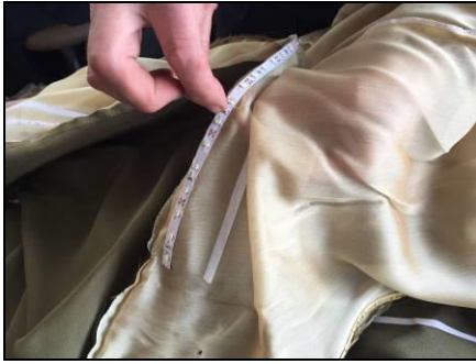
Figure 8. Sewing flexible leds
